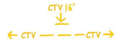
(xv) In areas where cables are spliced, the facilities should be located individually as far as possible on both sides of the splice. When the signal is distorted due to the near proximity to the splice a circle with "SP" should indicate the area of distortion or "splice pit".
